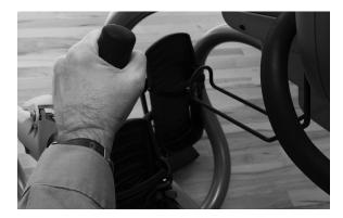
2. To lock the arms and pedals, push down on the StrideLock lever. Verify that the lock is engaged by pushing or pulling the upper arm grip.
